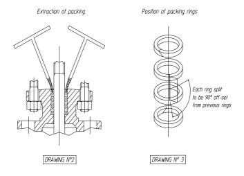
**<u>C</u>** Each ring should be firmly compressed into position before the next ring is added. Rings should fit snugly into the stuffing box. Install the gland and the gland flange and secure with the gland nuts, tighten the nuts uniformly and only to the extent needed to prevent leakage (check it in service).
