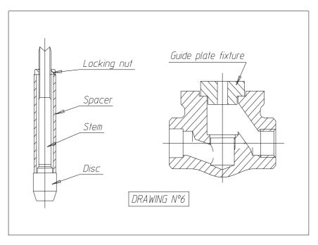
The valve handwheel con then be re-attached to the stem and used as a convenient handle when re-lapping the seats.
