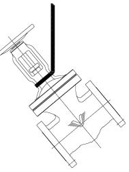
С Transport, unpack and store carefully not to scratch the surfaces of flanges or gasket and not to allow inclusion of hazardous matters into the valves. Wooden plate or plastic caps should not be removed until the piping installation.
